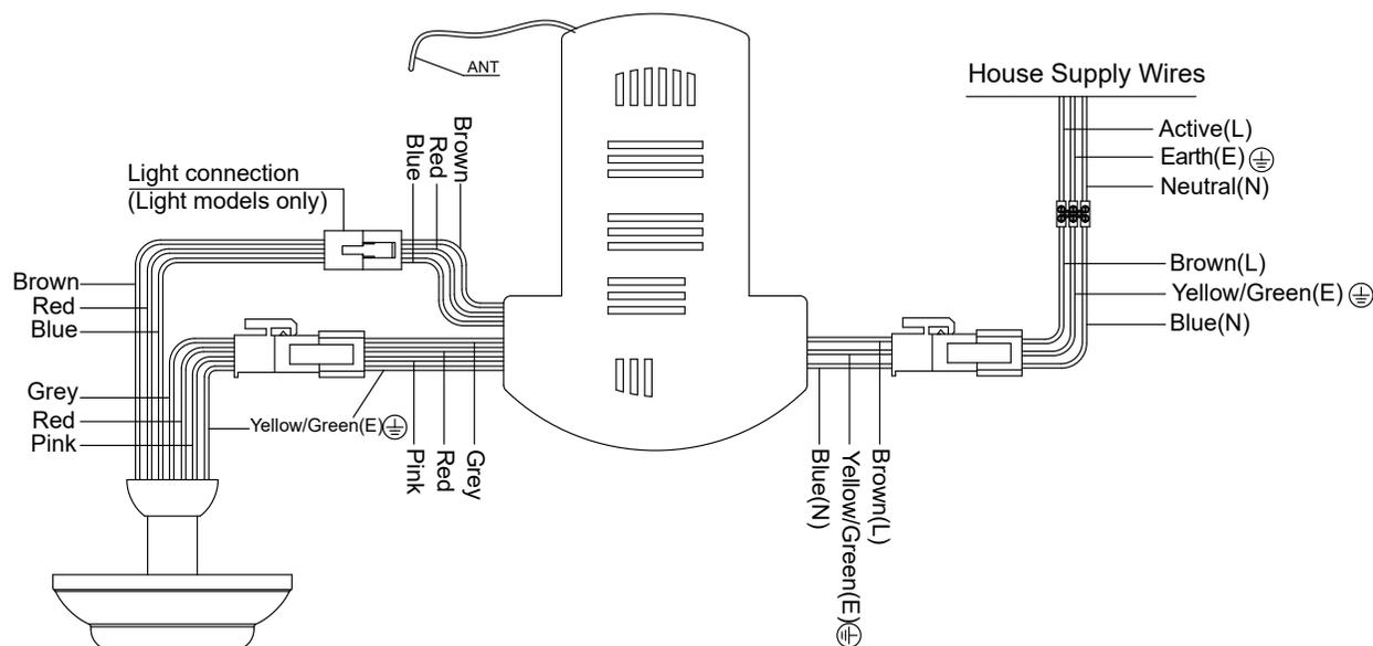
**Note:** For safe use of this fan, and all-pole disconnection **MUST** be incorporated into the fixed wiring in accordance with the wiring rules. As outlined in clause 7.12.2 of AS/NZS 60335-1 for meeting the minimum electrical safety of this standard. A single-pole switch also must be placed in the same room as the fan as per local wiring regulations AS3000.
